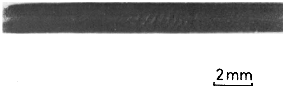
Fig. 9. Example of skin/core morphology. Sample A molded at 220°C.
